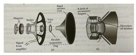
The force is always perpendicular to both the conductor and the field, with the direction determined by the same right-hand rule we used for a moving positive charge. Hence, this force can be expressed as a vector product, just like the force on a single moving charge. we represent the segment of wire with a vector I along the wire in the direction of the current, then force **F** on this segment is
